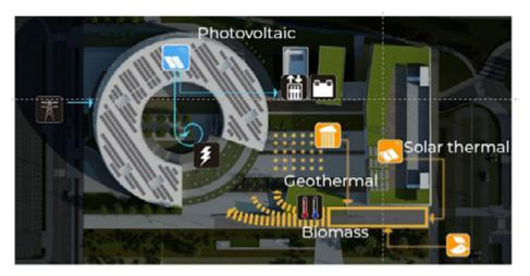
${\bf Blue-the\ origin\ and\ consumption\ of\ electrical\ energy; orange-the\ origin\ of\ the\ thermal\ energy\ distributed\ through\ the\ District\ Heating-Cooling.}$
