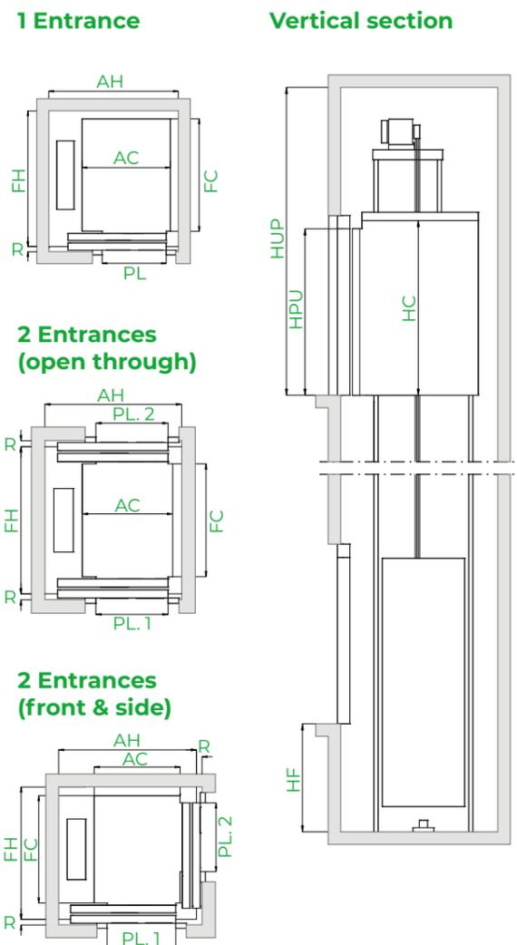
\*Note: The diagrams are for guidance only. Dimensions for 1 entrance. Car width and depth variable, in 5 mm increments. For simplification, table samples show increments of 100 mm.
