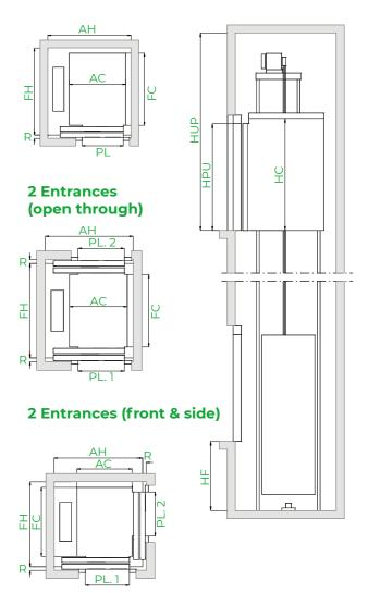
\*Note: The diagrams are for guidance only. Dimensions for 1 entrance. Car width and depth variable, in 5 mm increments. For simplification, table samples show increments of 100 mm.
